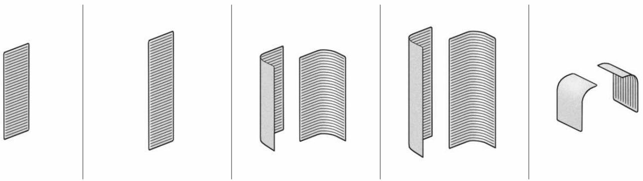
**The furniture system is distinctive for the use of five basic elements (panels) which are unified with respect to dimensions and design, allowing for easy configurability of all types of furniture. The flexible elements offer an opportunity to arrange the office interior with the use of armchairs, sofas, desks, partition walls and phone booths.**
