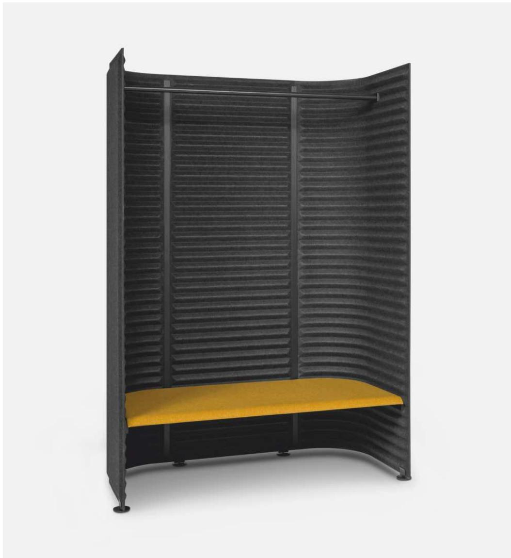
A unique feature of SoundRoom is the use of light polyester felt. The non-woven fabric covers on both sides a honeycomb-shaped cardboard core with hexagonal cells. The resulting element, produced in the process of thermoforming, is a lightweight, extremely rigid and visually attractive panel which is pleasant and warm to the touch. The panels have a characteristic wavy shape on the inner side and are flat on the outer side.
